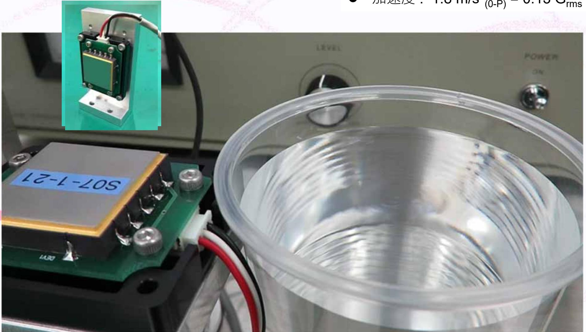
理論限界 =  $0.5 \times (1.9108 \text{ g} + 47.9 \text{ mg}) \times 2\pi 95\text{Hz} \times 540\mu\text{m} \times 2.5\text{m/s}^2 = 789 \mu\text{W}$
